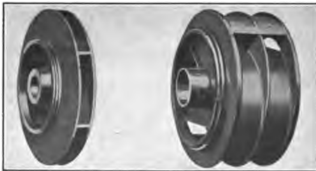
Enclosed side suction impeller.
